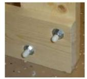
are 'small shelf caps' that are used on cut ends of metal shelving. These are available at most stores that sell 'do it yourself' metal shelving and they cost about \$0.06 each when bought in a bulk package of 100.
