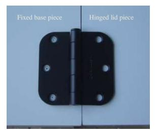
Connect the hinge to the fixed base piece first. It is recommended that care be taken when attaching the hinges to both pieces. After the hinges are in place, mark the center of the screw holes with a pencil, then use a punch to indent the desk top pieces, and then predrill a small and shallow hole for each screw. Taking this care will better ensure that the hinges will be in the proper place when the screws are tightened. Attach both hinges to the fixed base piece then to the hinged lid piece.
