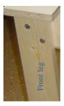
After front legs are attached, attach back 2 legs in a similar manner. Again line up the back legs ensuring that they are square with the support box AND also lined up adjacent to
