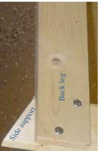
the 'shorter corner' (~  $15 \ 1/8$ ") of the side support pieces. Drill <sup>1</sup>/4" holes for 2 carriage bolts in diagonal pattern ensuring that there is sufficient room inside of support box to work with the flat washers and nuts that must be attached to bolts. Again insert bolts from outside such that washer and nuts are inside desk enclosure. See picture above.
